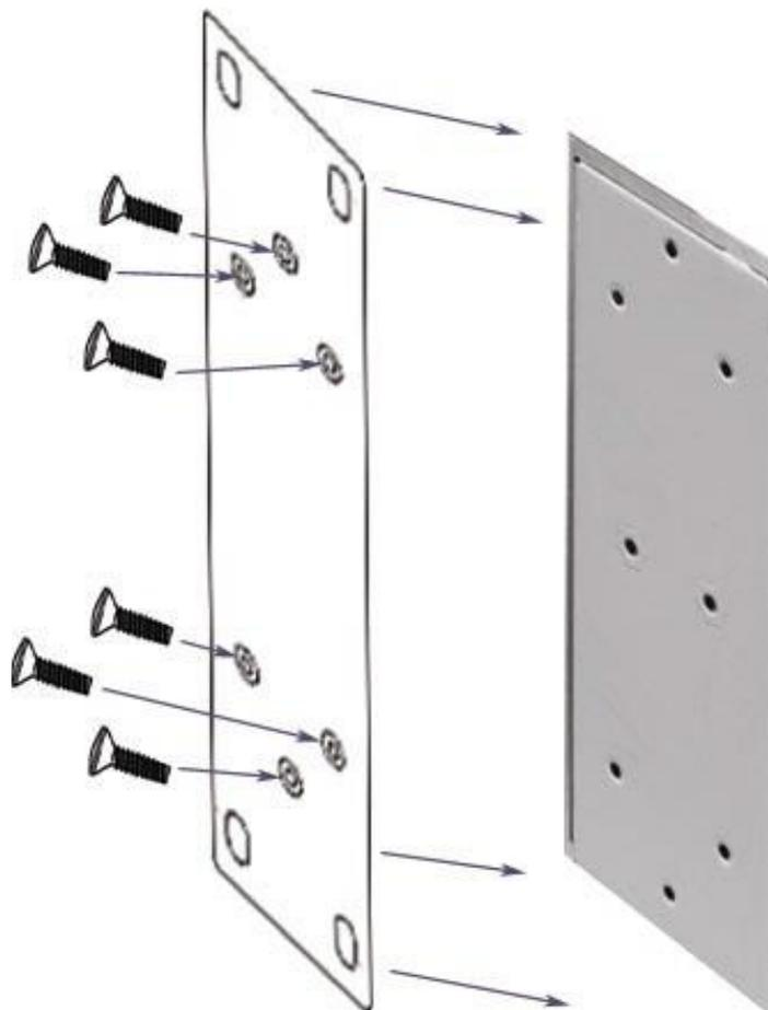
Screws to mount the wall mount plate on the Industrial switch.
