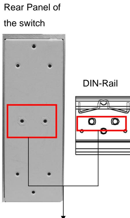
1. Use the screws to mount the DIN-Rail on the industrial switch
