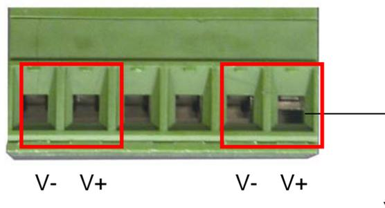
1. Insert the positive and negative wires into the V+ and V- connector on the terminal block connector.
