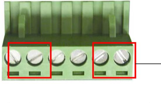
2. Tighten the wire-clamp screws to prevent the DC wires from becoming loose.
