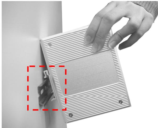
2. Then, lightly push the button of DIN-Rail into the track.
