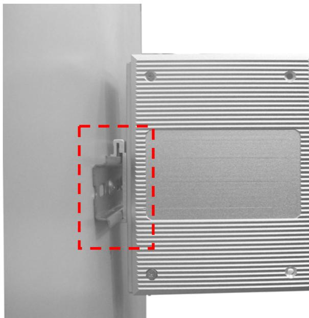
3. Check the DIN-Rail is tightly on the track.
