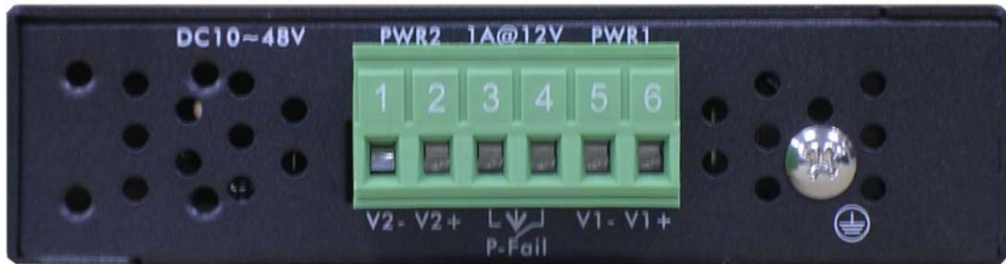
Top Panel of the 5 10/100TX Industrial Switch
